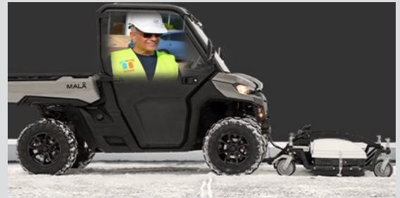
Left: Maya's experts are measuring the surface with the GRP-HDR tool and a base-rover GNSS set up for positioning
